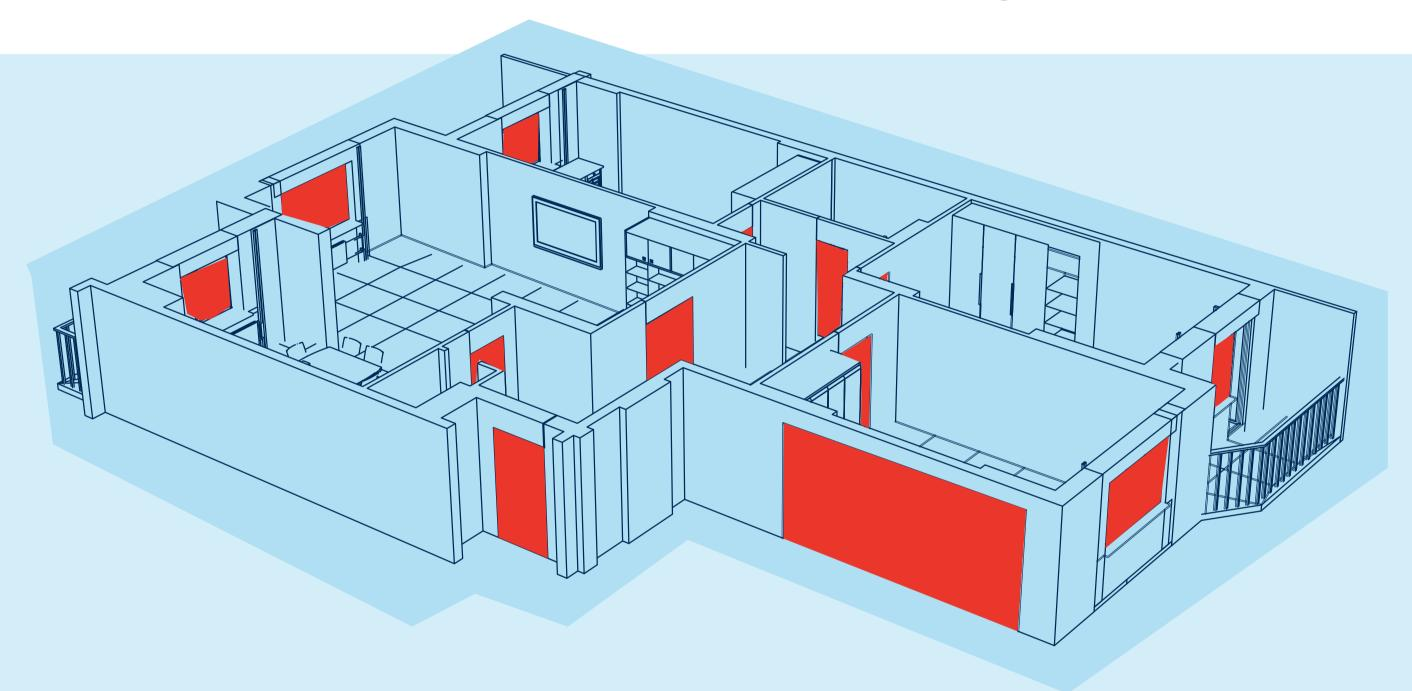
High winds place homes under intense pressure. Wind entering the home through an open or broken window, can create strong upward pressure on the roof. Rigorous scientific wind testing on a full-scale, 1,400-square-foot single-story home at the IBHS Research Center reveals closing interior doors helps compartmentalize the pressure inside a home into smaller areas reducing the force on the roof by 30%, which gives the roof a better chance of staying intact.
